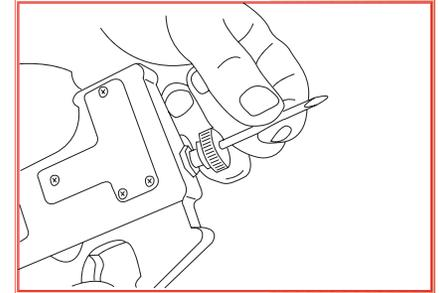
2. Tighten the collet until the needle fits securely.
